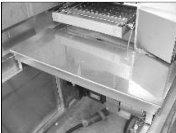
25. Glaze reservoir installed.
